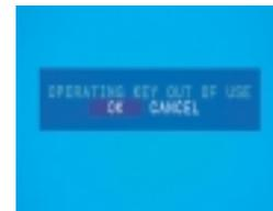
Using a setting on the on-screen menu, you can disable the operation of all of the controls on the top and rear panels of the projector. This setting can only be
