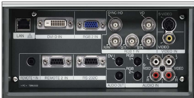
Terminals include an HDCP-compliant DVI-D input connector
